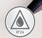
The Oslo panel heaters are suitable for all locations, and approved for use in bathrooms with an IP24 splash proof rating. This design feature means that the appliance has the ability to be easily and safely installed into most household applications.
